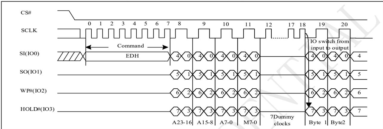
Note: 1. Hi-impedance is inhibited for the mode clock cycles. 2. M[5-4] = (1,0) is inhibited.
