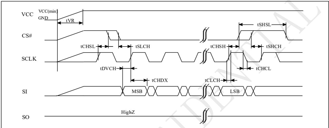
**Figure 5-9 Power-up Timing**
