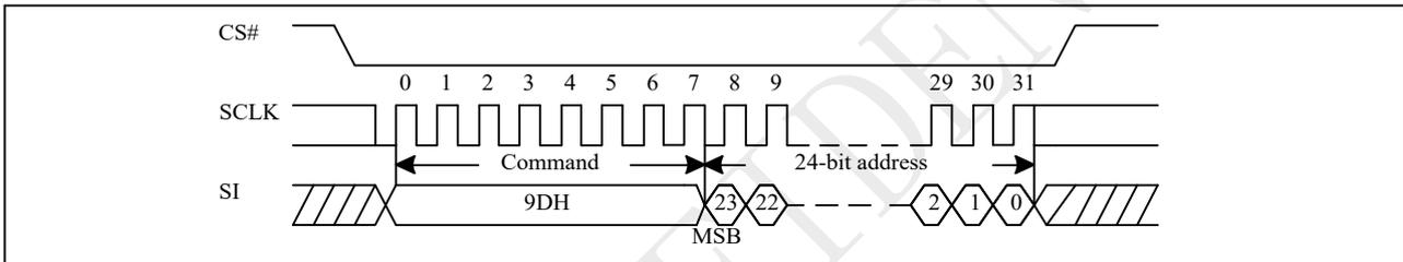
**Figure 10-37a Buffer to Main Memory Page Program Sequence (QPI)**
