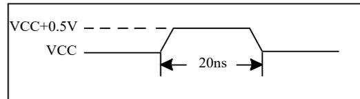
During DC conditions, input or I/O signals should remain equal to or between VSS and VCC. During voltage transitions, inputs or I/Os may negative overshoot to -0.6V or positive overshoot to VCC + 0.5 V, for periods up to 20 ns.
