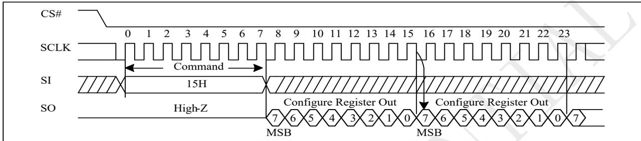
Figure 10-6a Read Status Register (RDCR) Sequence (QPI)
